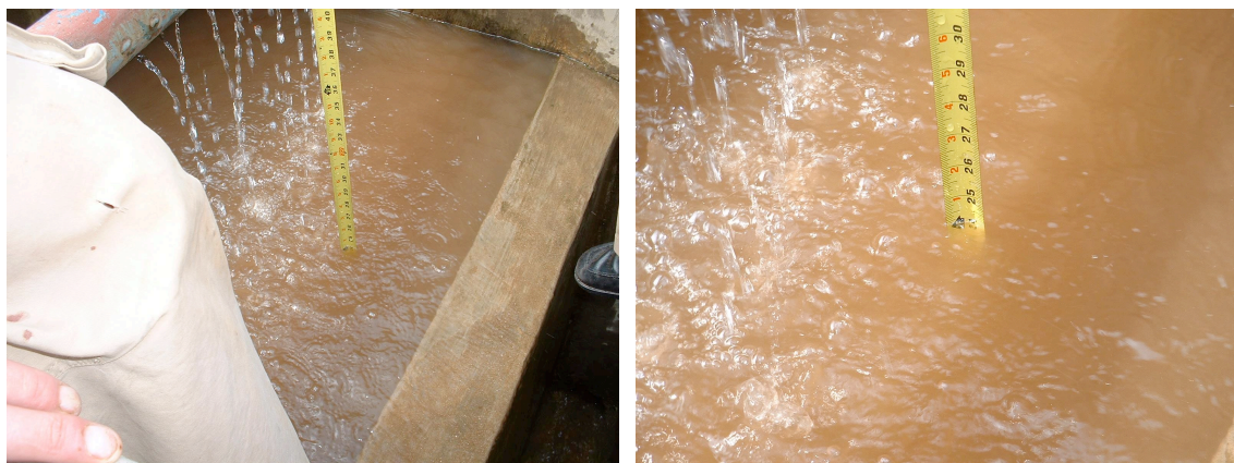
Measurement of the maximum freeboard during the backwash process. The end of the tape is resting on top of the sand layer; the waterline is at 24".
